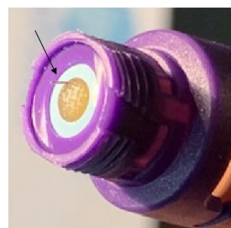
Figure 4. Needle Stump Broken, shown by the Arrow, Remaining Within the Insulin Pen Rubber. When a New Needle is Screwed onto This Pen, Some of the Insulin Leaks Outside Through the Needle Stump, Thus Changing the Injected Dose (Personal Archive)
